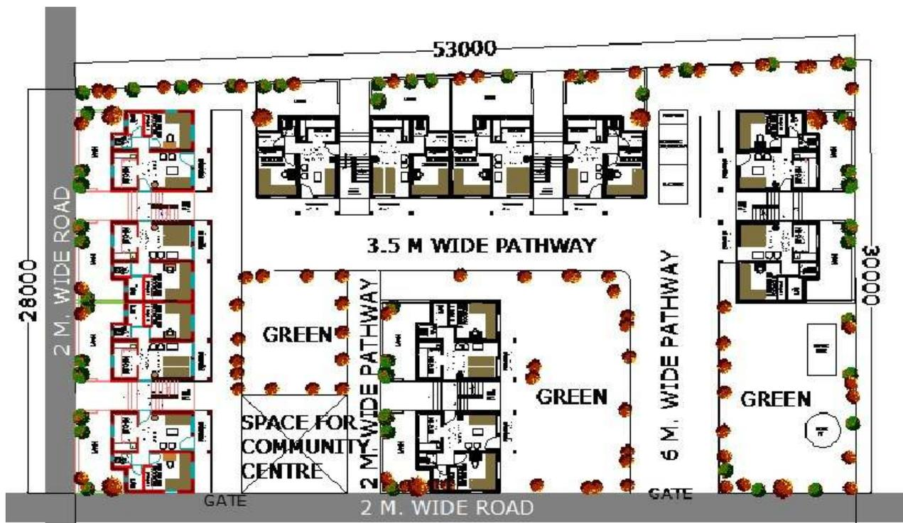
Figure 1: Site layout showing primary C shaped circulation loop with the entrances to the individual buildings.
