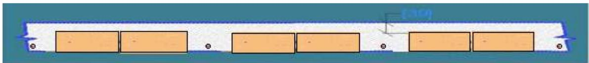
**Filler slab with a pair of Bricks as filler.**
